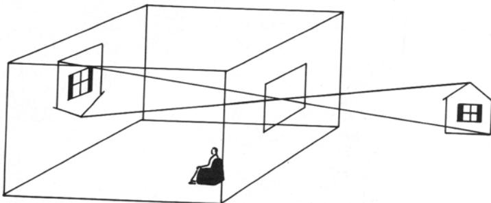
**The optical principle on which photography is based.**
