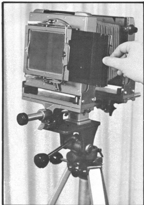
The flexibility comes from the bellows. You can raise and lower the lens mount. And the film back. Plus, you can tilt both parts. The bellows just goes along with whatever you're doing.
