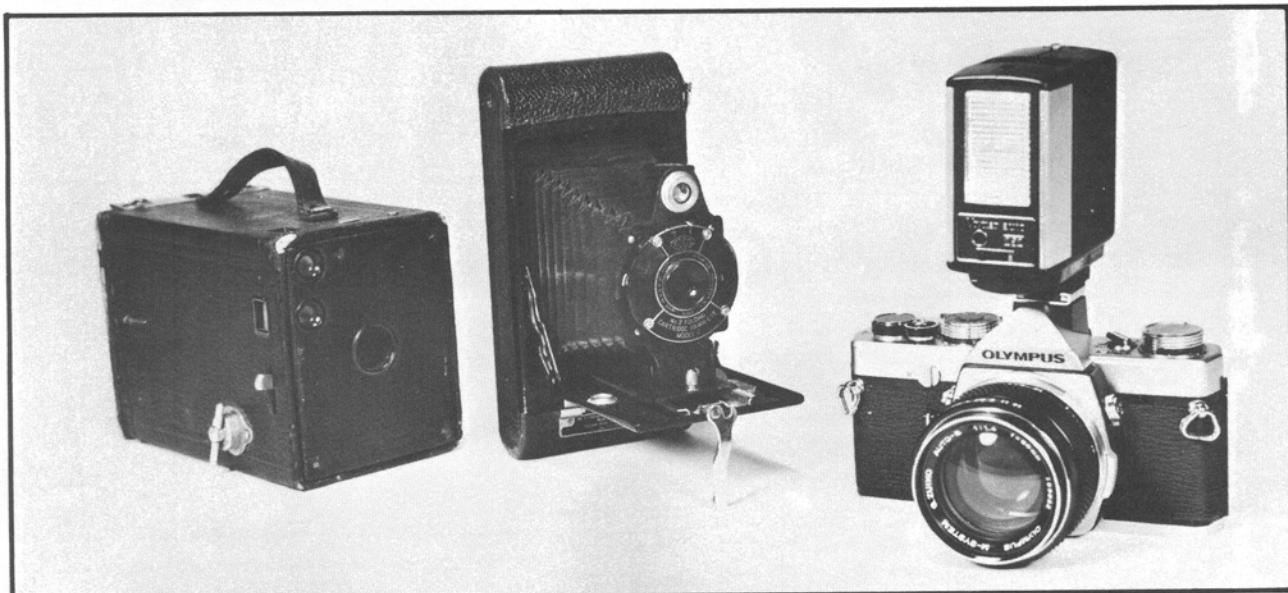
Three steps in the evolution of the camera — an early box camera, an early folding camera, and a modern miniature camera.
